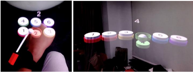
Figure 3: Air Hit shot through the lens. Left picture shows the two-row layout, right picture shows the buttons placing far away from the user.
